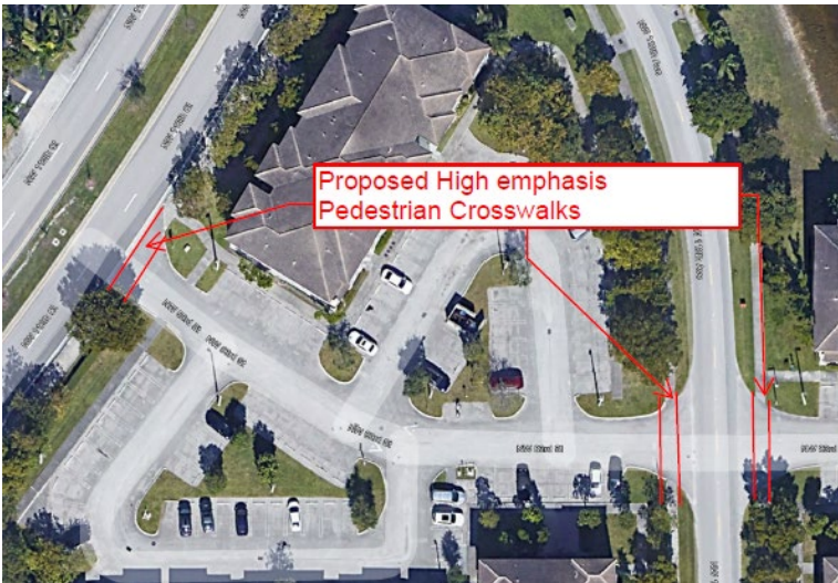
Location 5- NW 109 Ave and NW 88 St: Proposed high-emphasis pedestrian crosswalk and new ramp.
