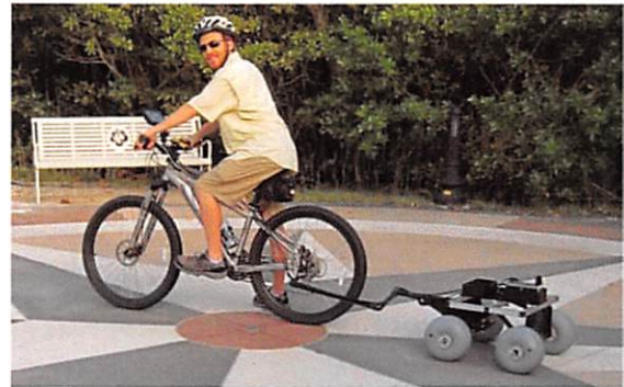
Our wheeled right-of-way assessment cart can take photos, slope, and GPS readings, allowing quick assessment of miles of sidewalks and paved trails.
