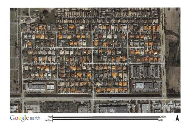
The Vanderbilt Park is bound by NW 25<sup>th</sup> Street to the South, NW 97<sup>th</sup> Ave to the East, NW 28<sup>th</sup> Terrace to the North and NW 102<sup>nd</sup> Ave to the West. As part of traffic calming study, recommendation of traffic calming devices were identified to solve cut through and speeding problems and meet the consensus of the neighborhood.
