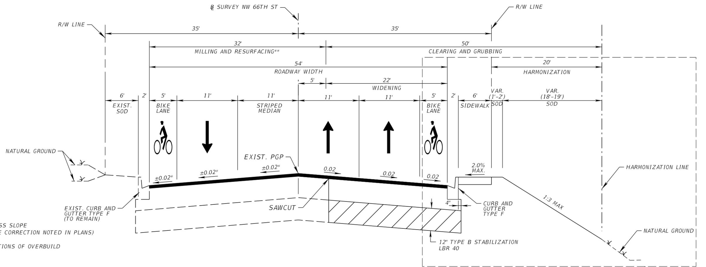
\* MATCH EXISTING CROSS SLOPE (UNLESS CROSS SLOPE CORRECTION NOTED IN PLANS)
