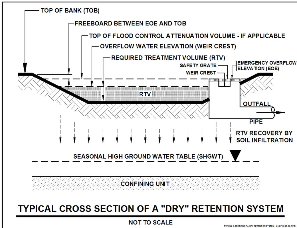
Figure 6-20 – Typical Cross-Section of a “DRY” Retention Pond
