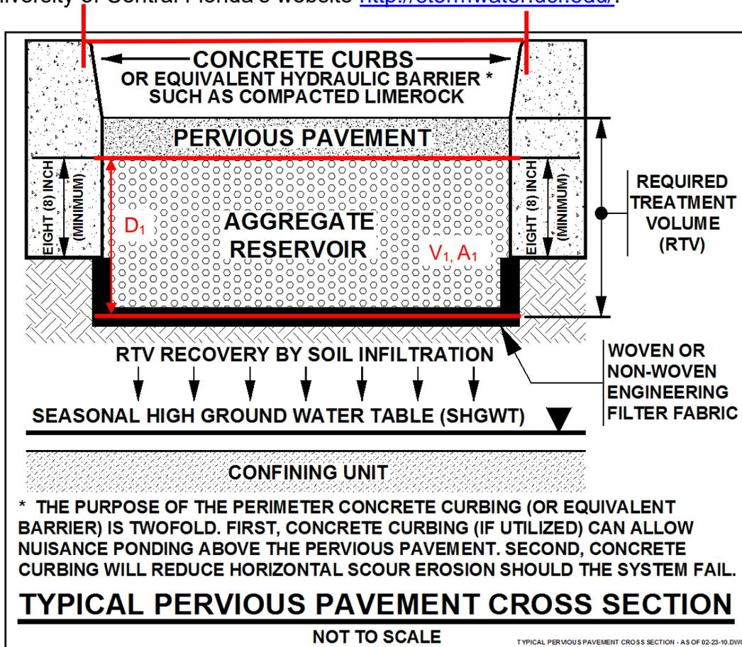
Figure 6-18 – Typical Pervious Pavement Cross-Section
