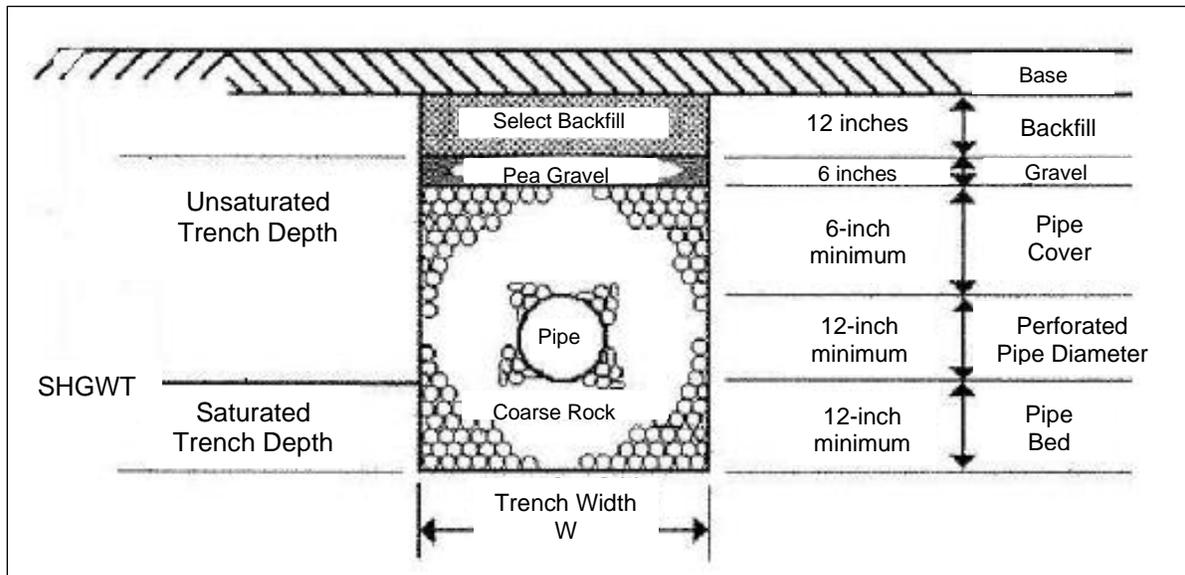
Figure 6-12 – Generic “WET” Exfiltration Trench
