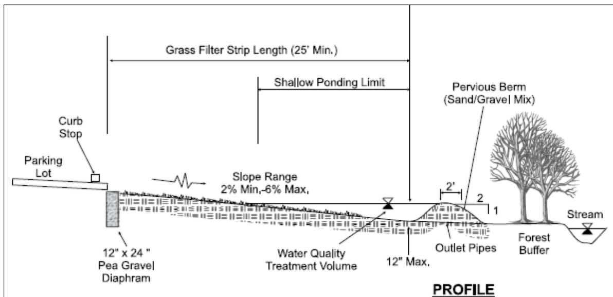
Figure 4-5 – Typical Profile of a Filter Strip
