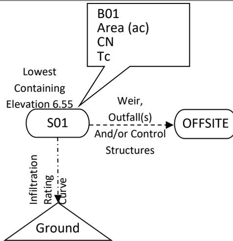
Figure 8-5 - Node-Link Schematic for Post Developments Condition Model
