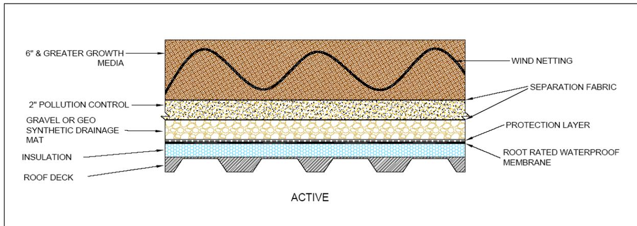
Figure 6-16 – Intensive Green Roof Section (Usually Active Function)
