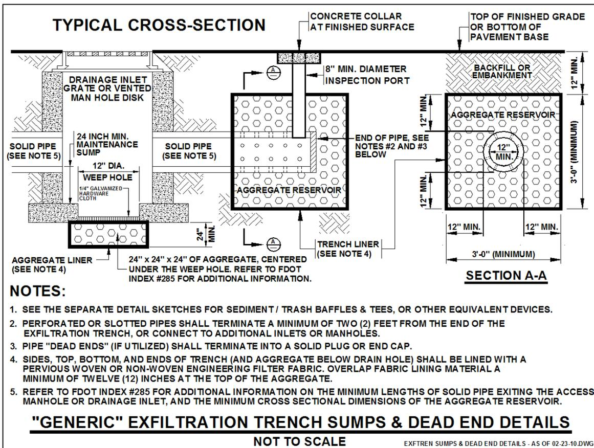
Figure 6-14 – Typical Exfiltration Trench Sumps and Dead End Details
