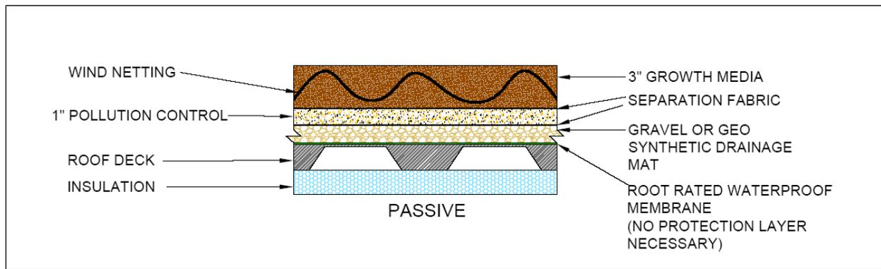
Figure 6-15 – Extensive Green Roof Section (Usually Passive Function)
