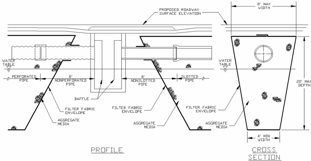
Figure 4-7 - Typical Exfiltration Trench
