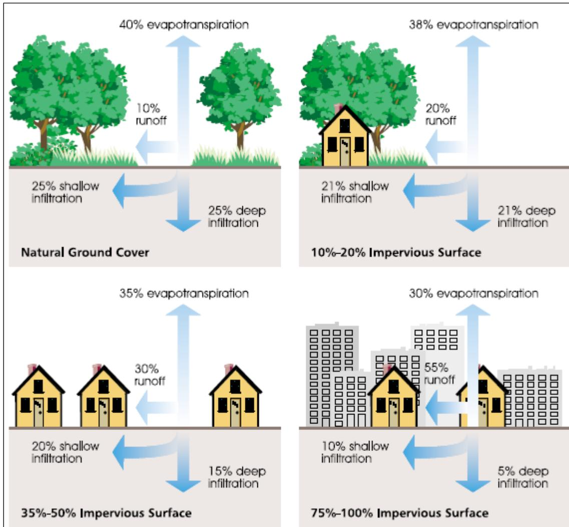
Figure 5-1 – Surface Runoff Variability with Increased Impervious Surfaces
