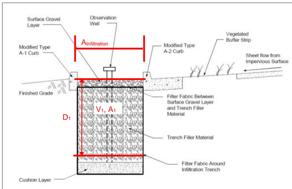
Figure 6-10 – Infiltration Trench Conceptual Drawing
