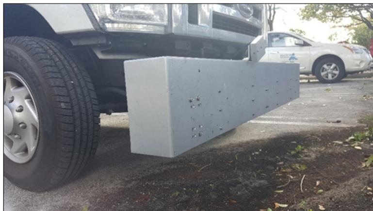
*Figure 4. Inertial Roadway Profiler Sensor Bar*
