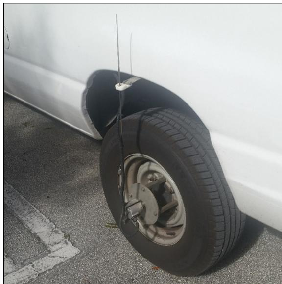
*Figure 5. Inertial Profiler Distance Measuring Equipment*
