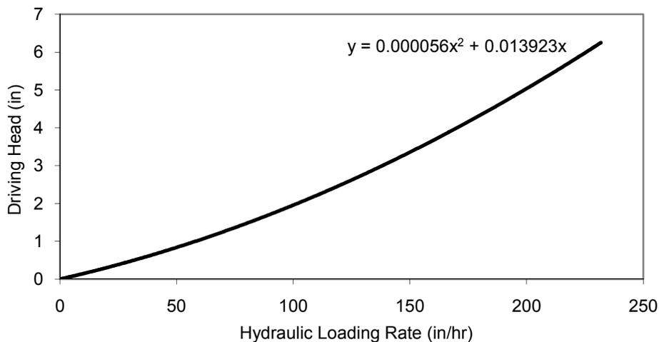
**Figure 11 - Hydraulic Loading Characteristics of the Filter Media**
