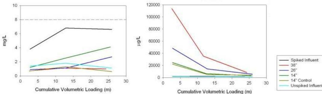
**Figure 7.** Ion exchanges for a coconut-hull GAC-sand mixture as a function of column depth for nitrate (left) and potassium (right).
