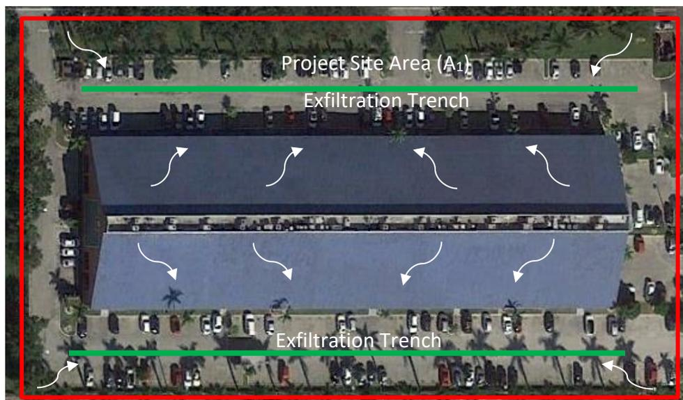
Figure 7-1 - Area Attributed to an Exfiltration Trench Length
