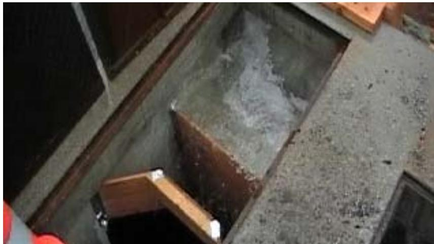
**Figure 1. View of Inlet/Outlet Bay and a portion of the StormFilter Bay at 59 l/sec (2.1 cfs), 27 seconds into “instant-on” hydraulic test. Note that StormFilter Bay is still empty which indicates that the system is still in the process of filling.**
