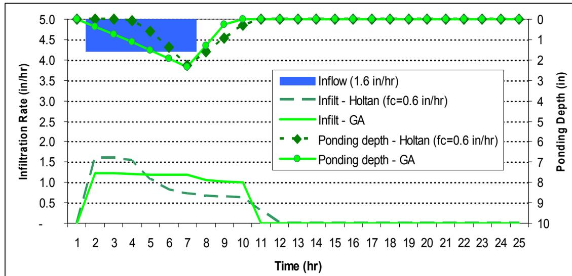
**Figure 2. Comparison of the infiltration simulation results using Holtan-Lopez and G-A methods.**
