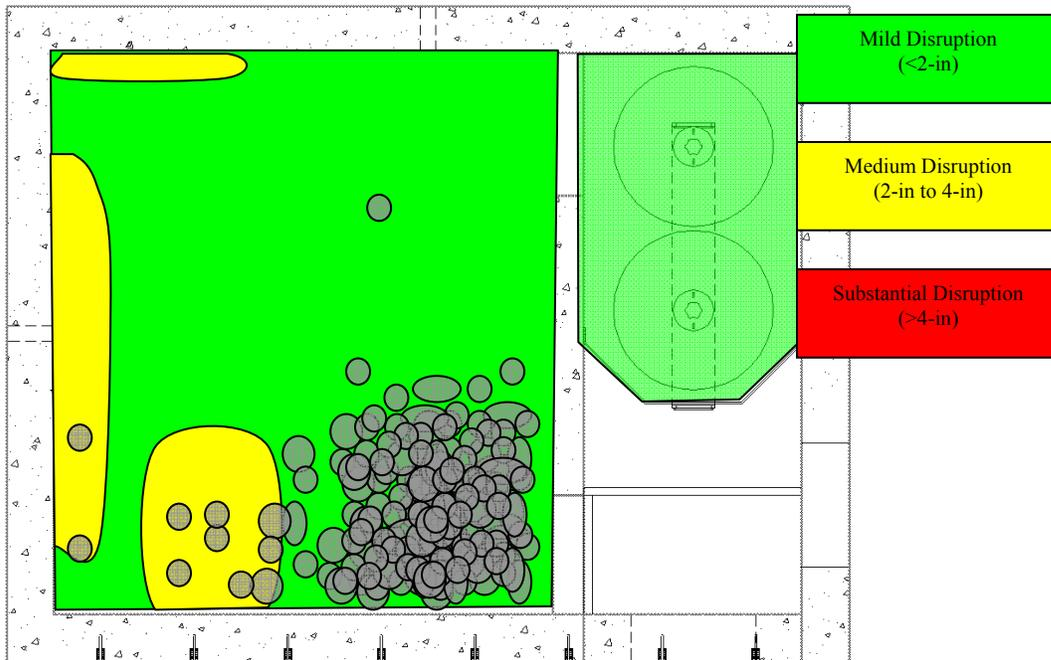
**Figure 9. Surface disruption pattern for Trial 7, which involved instantaneous peak flows and 5 cm - 15 cm cobble armor 16 cm deep in an approx. 0.37 m<sup>2</sup> area.**
