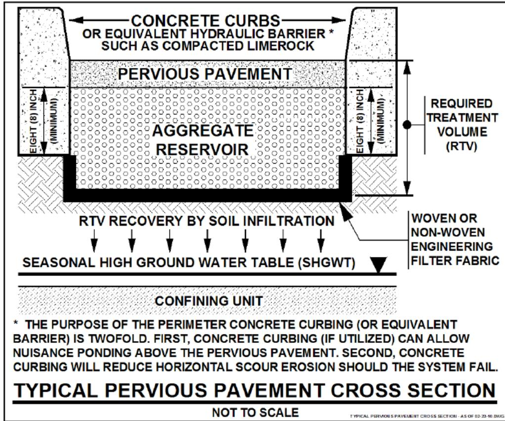
Figure 4-9 - Typical Pervious Pavement Cross-section
