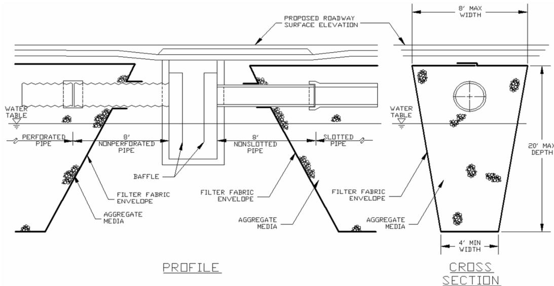
Figure 4-7 - Typical Exfiltration Trench
