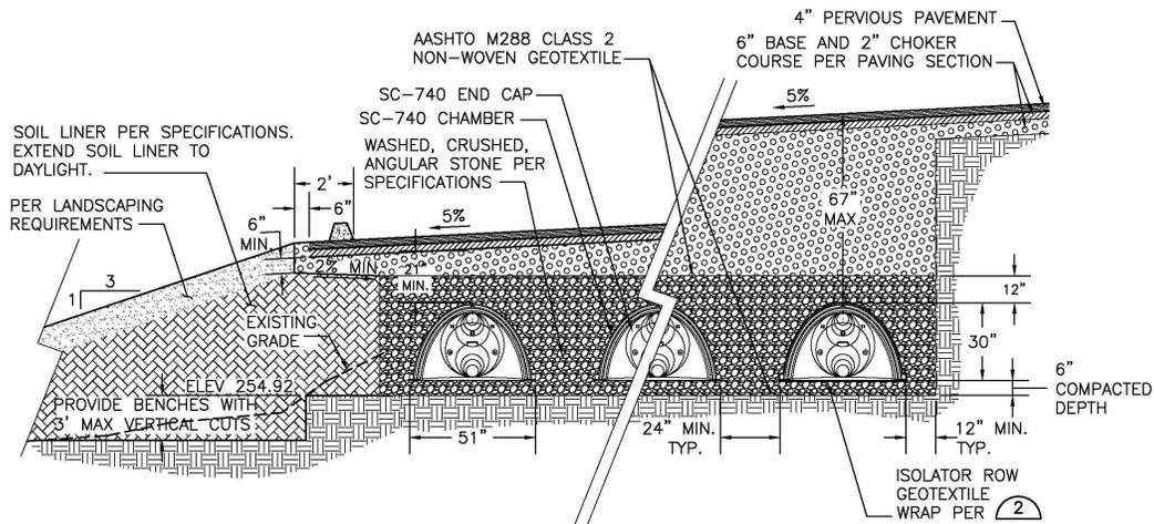
**Figure 1. Integrated pervious asphalt and detention system**
