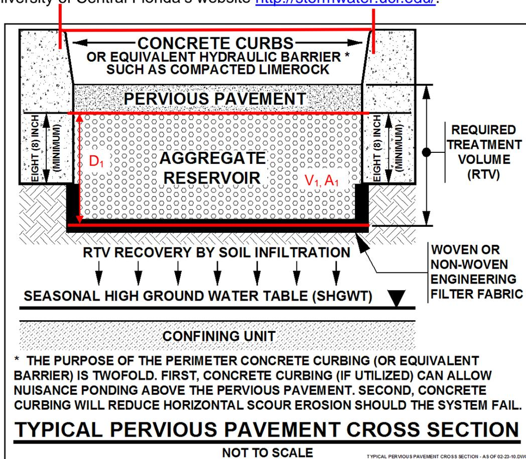
Figure 6-18 – Typical Pervious Pavement Cross-Section
