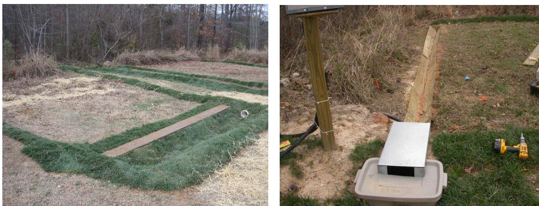
Figure 2. Level spreader, recollection trough, and weir box.
