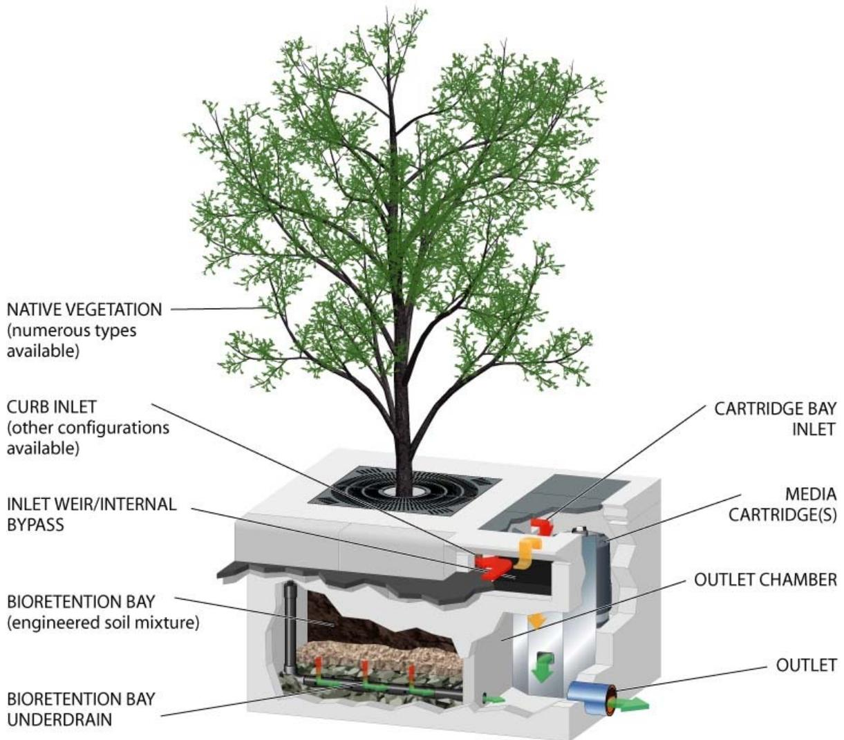
**Figure 1 – UrbanGreen™ BioFilter, Basic Operation & Components**
