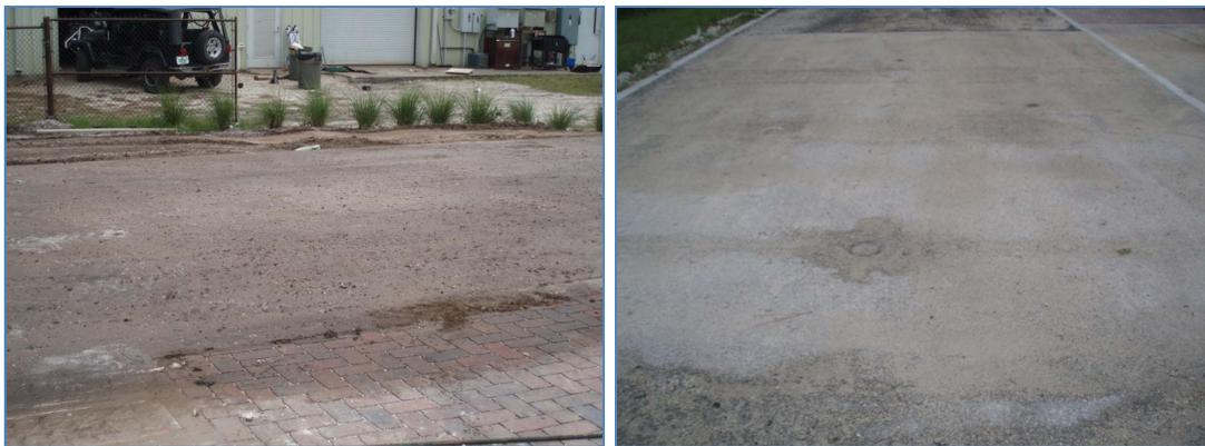
Figure 2 (a) Sandy sediment loaded surfaces (b) Fine limestone dust loaded surfaces
