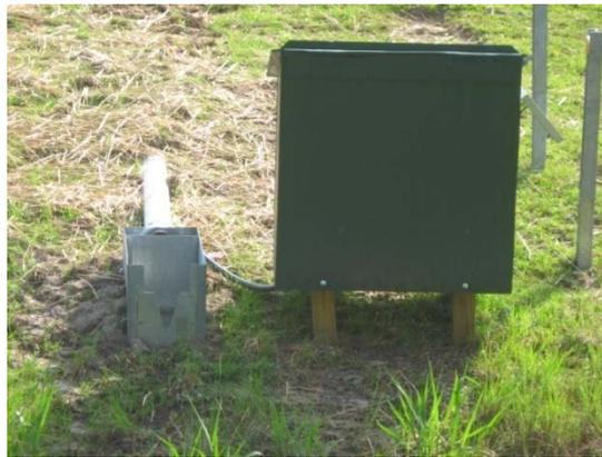
Figure 7. Weir Box for sample collection at edge-of-pavement and VFS outlet.
