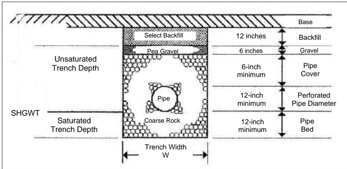
Figure 6-12 – Generic “WET” Exfiltration Trench
