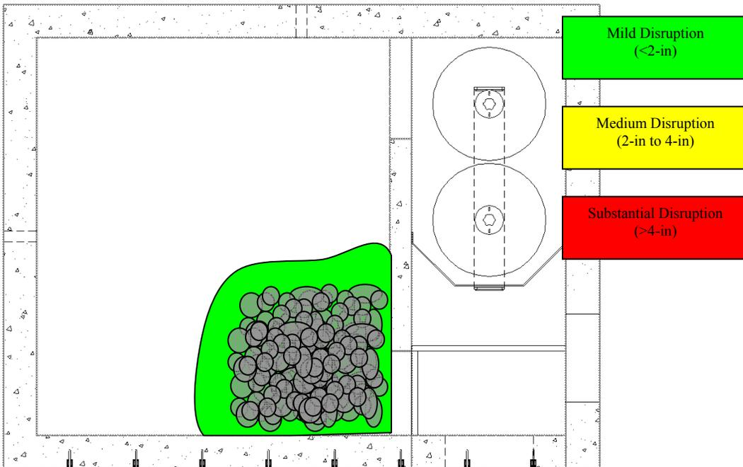
**Figure 8. Surface disruption pattern for Trial 6, which involved 5 cm - 15 cm cobble armor 16 cm deep in an approx. 0.37 m<sup>2</sup> area.**
